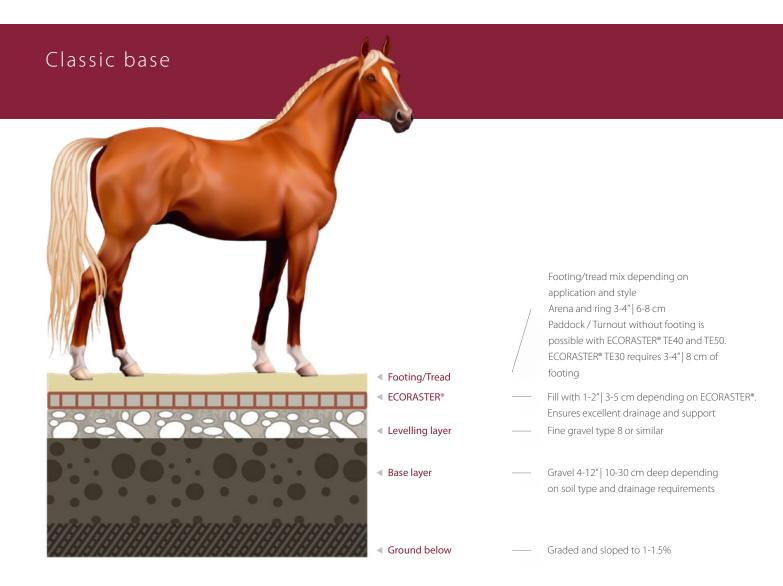
Ground Below Grade and slope 1-1.5% depending on requirements
